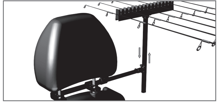
2. Adjust the Foam Tip Holder (7) height for easy loading
