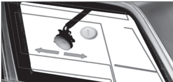
5. IMPORTANT! Do not place suction mounts on the gridlines if applied to the window. Gridlines will prevent the suction mounts from maintaining a vacuum.
